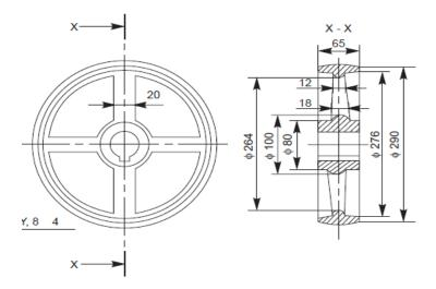
2 Draw the following figure in first angle projection method.
